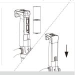
Install two pcs DD batteries, slide down and close the battery cover.
